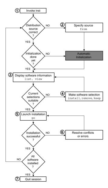
Figure 5-1 Summary of the Installation Procedure
