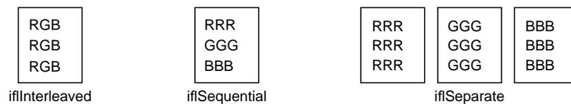
**Figure 2-4** Pixel Data Ordering for an RGB Image
