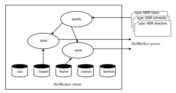
Figure C-6 Saving Two Filesystems in Parallel
