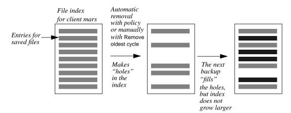
Figure 7-3 Removing a Cycle From an Index
