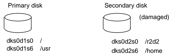
Figure A-3 Secondary Disk Damaged
