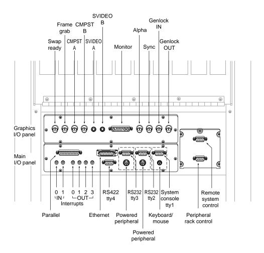
**Figure 2-6** RE<sup>2</sup> and Main Graphics I/O Panel Connectors
