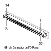
**Figure 4-5** 68-Pin Connector Pin Numbering
