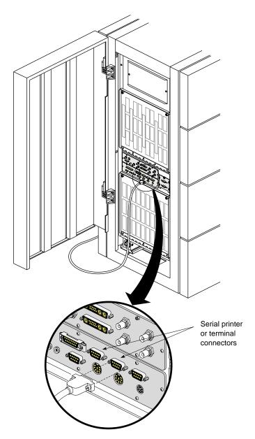
**Figure 4-7** Connecting a Serial Printer or ASCII Terminal
