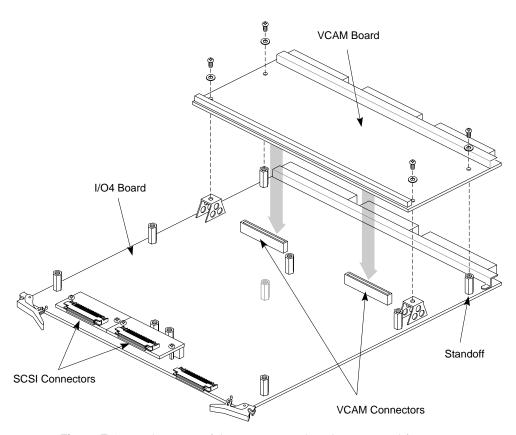
Figure E-1 Placement of the VCAM Board on the IO4 Board for CC2
