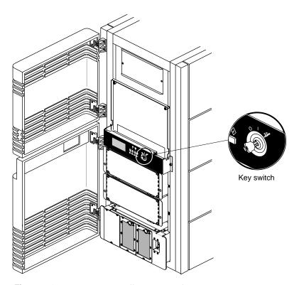
Figure 3-10 System Controller Key Switch
