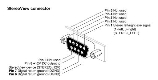
Figure 2-8 InfiniteReality StereoView Connector Pinouts
