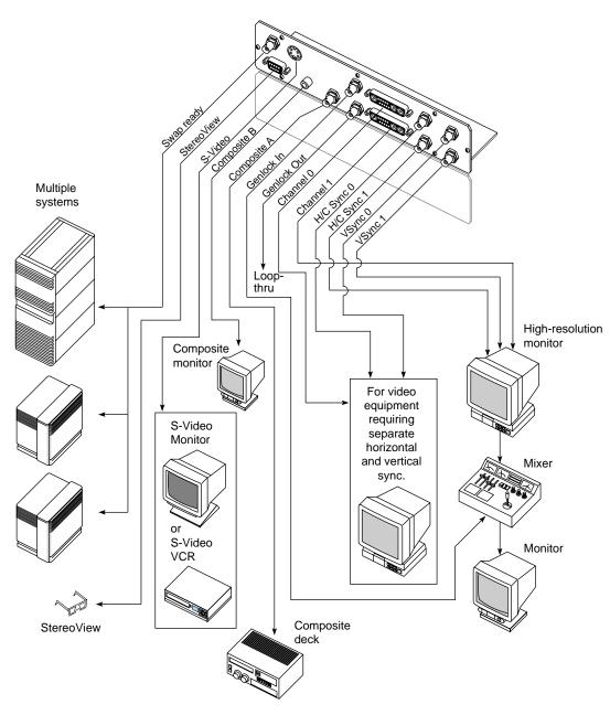
**Figure 3-3** InfiniteReality Video Peripherals Connection Example
