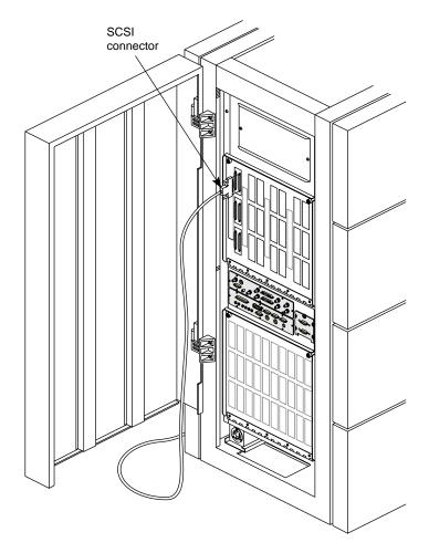
Figure 4-4 Connecting an External SCSI Device
