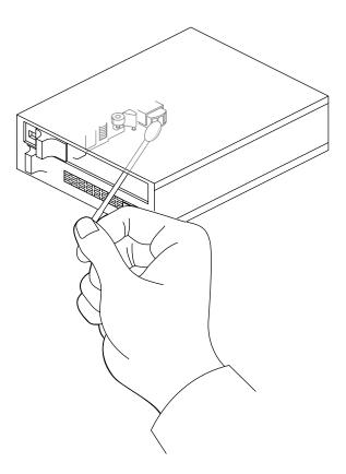
Figure B-5 Tape Head Cleaning
