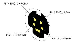
Figure 2-9 InfiniteReality S-Video Connector Pinouts
