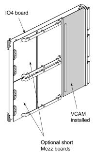
Figure D-1 IO4 with VCAM
