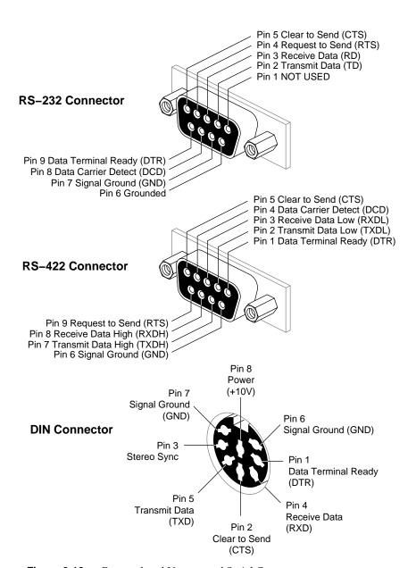
Figure 2-12 Powered and Unpowered Serial Connectors
