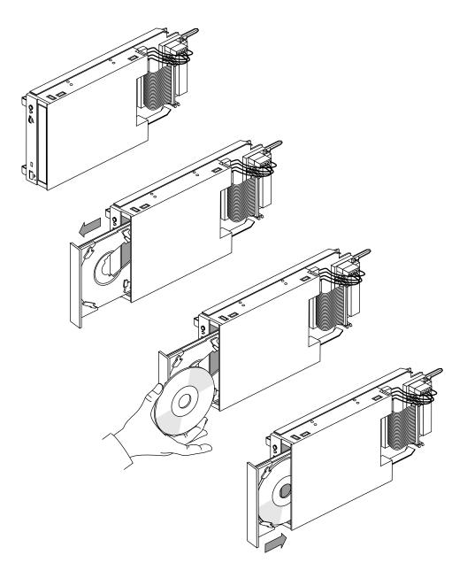
**Figure 4-6** Loading a Disc Into the CD-ROM Drive
