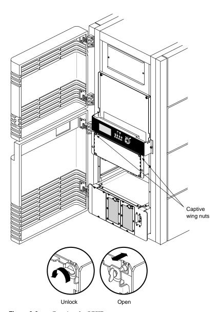
**Figure 3-6** Opening the SCSIBox
