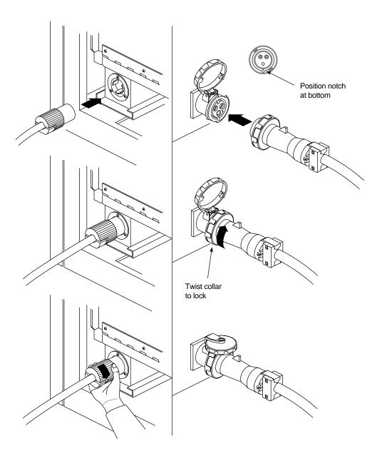
**Figure 3-8** Connecting the System Power Cable
