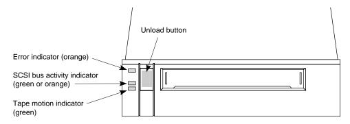
**Figure B-1** 8-mm Tape Drive Front Panel
