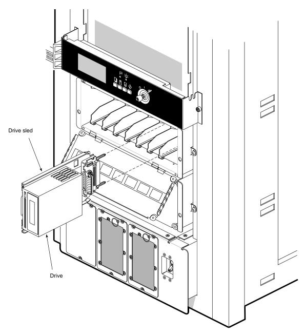
Figure 3-7 Installing a Front-Loading Device
