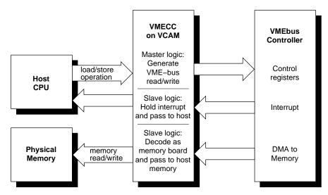
Figure E-3 VMECC, the VMEbus Adapter
