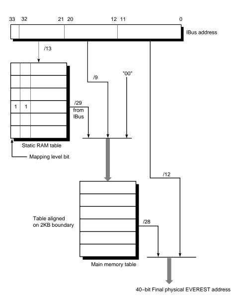
**Figure E-4** I/O Address to System Address Mapping
