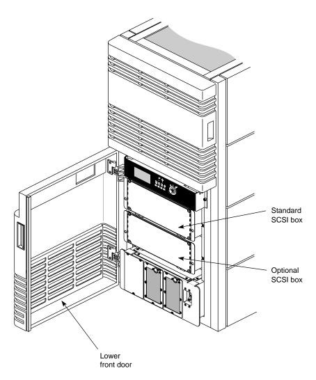
Figure 2-15 SCSIBox Drive Enclosures
