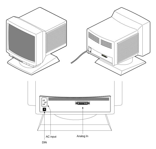
**Figure 3-1** 21-Inch Monitor Connectors
