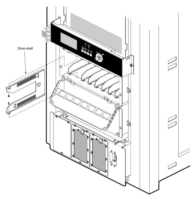
**Figure 4-3** Removing a SCSIBox Drive Shelf
