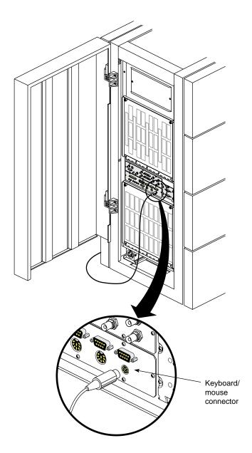
**Figure 3-5** Keyboard Connection
