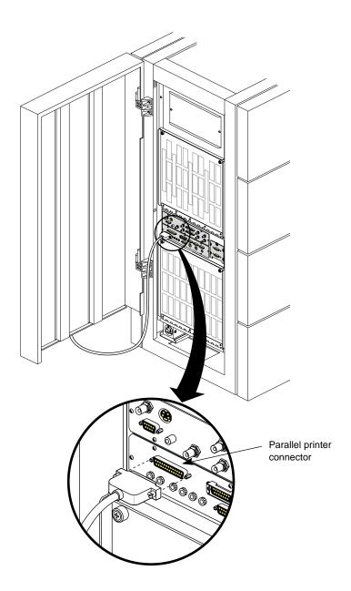
Figure 4-8 Connecting a Parallel Printer
