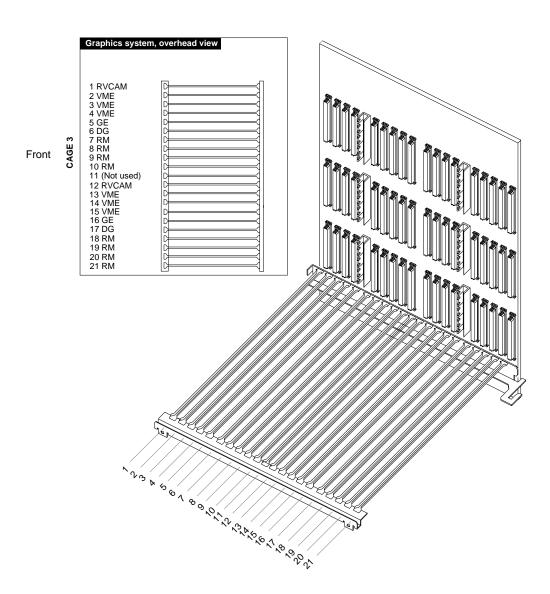
**Figure E-10** Rackmount RealityEngine<sup>2</sup> Card Cage 3 Slot Assignments
