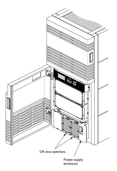
Figure 2-16 Power Supply Enclosure and OLSs
