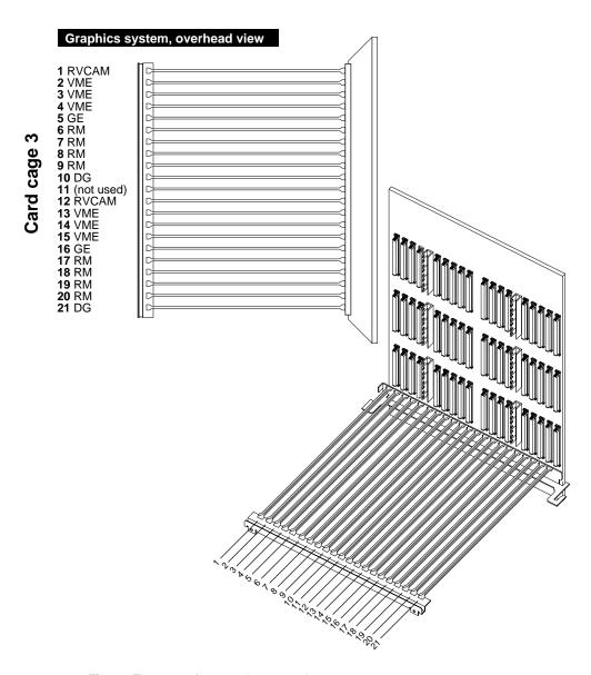
Figure E-7 InfiniteReality CC3 Slot Assignments
