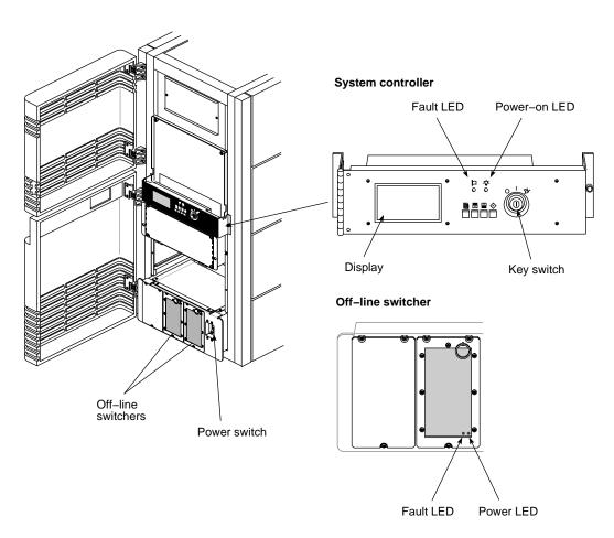
**Figure 2-3** Power Switches and Indicators
