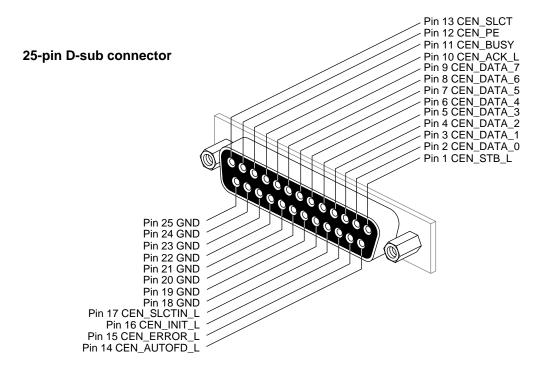
Figure 2-13 Parallel Port Connector Pinouts
