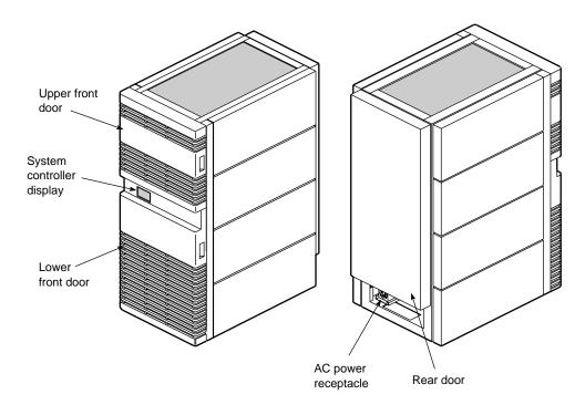
Figure 2-1 Chassis Front and Rear Views
