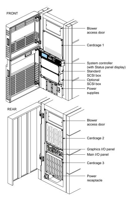
Figure 2-2 Onyx Rackmount Chassis With Doors Open
