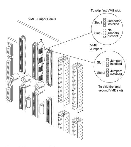
**Figure E-11** VMEbus Midplane Jumpers
