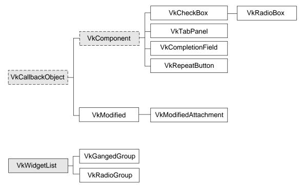
Figure 14-1 Inheritance Graph for the Miscellaneous ViewKit Input Classes
