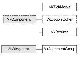
Figure 13-1 Inheritance Graph for the Miscellaneous ViewKit Display Classes
