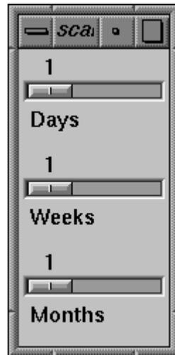
**Figure 4-3** Simple Example of a `VkSimpleWindow` Subclass
