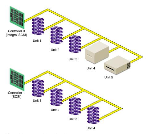
Figure 1-1 Controllers and Disk Drives
