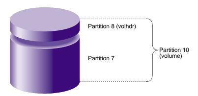
Figure 1-7 Partition Layout of Option Disks
