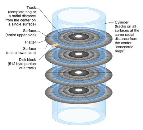
Figure 1-2 Physical Disk Structure
