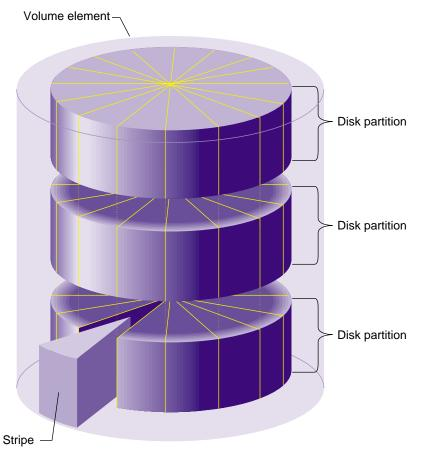
**Figure 6-9** Striped Volume Element Composition
