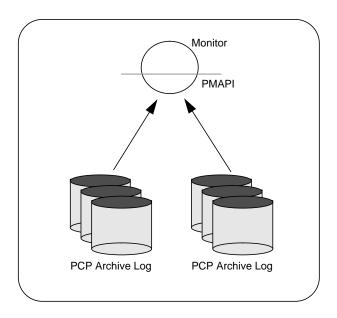
Figure 1-3 Architecture for Retrospective Analysis
