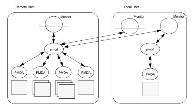
Figure 1-2 Process Structure for Distributed Operation
