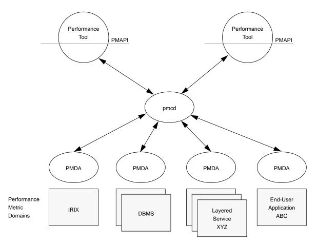
Figure 1-1 PCP Global Process Architecture
