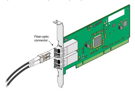
**Figure 1-2** Fiber-Optic Gigabit Ethernet Board
