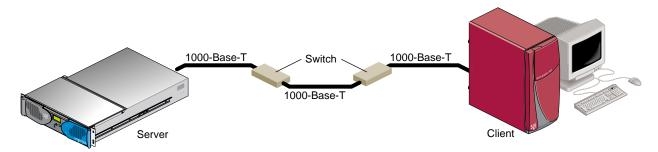
**Figure 1-5** Example of 1000-Base-T Configuration
