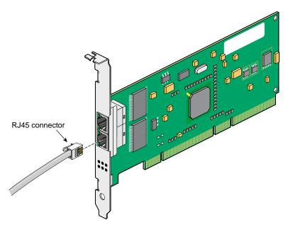
**Figure 2-2** Connecting the Copper Cable
