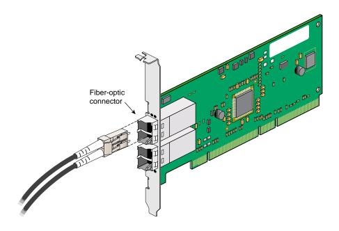
**Figure 2-1** Connecting the Fiber-Optic Cable
