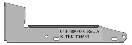
**Figure 1-1** Gigabit Ethernet Board Support Bracket
