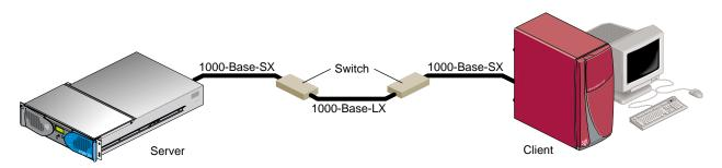
**Figure 1-4** Example of 1000-Base-LX Configuration
