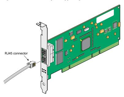
Figure 1-3 shows the dual-port Copper Gigabit Ethernet board.
