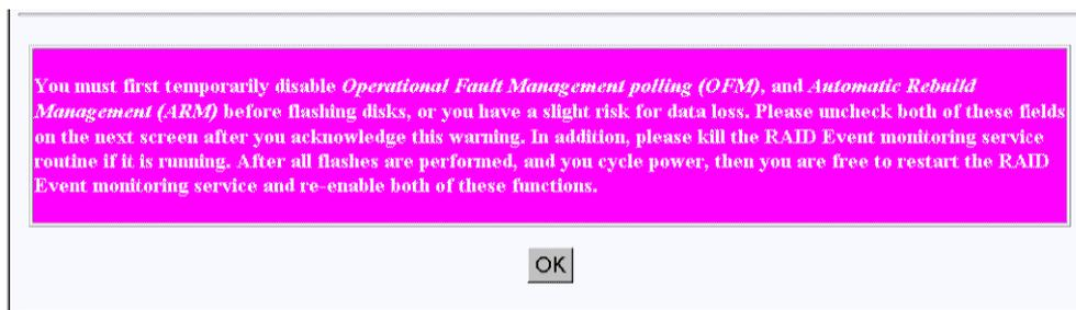
**Figure 3-63** Flash New Firmware Onto Supported Disk(s) Dialog Box
