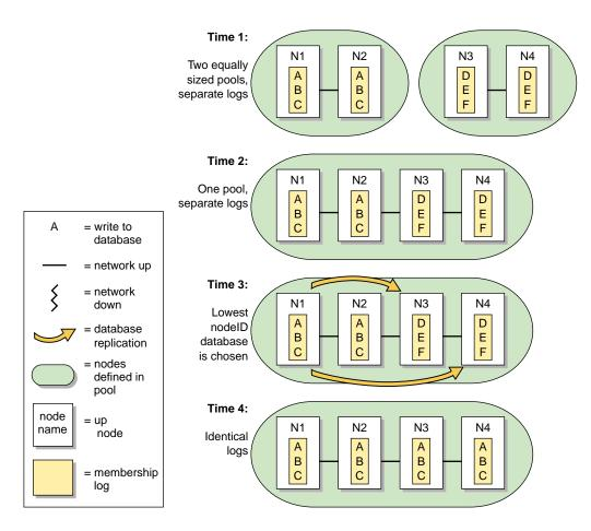
Figure 5-3 Equally Sized Pools are Joined: Lowest Node ID Log is Replicated
