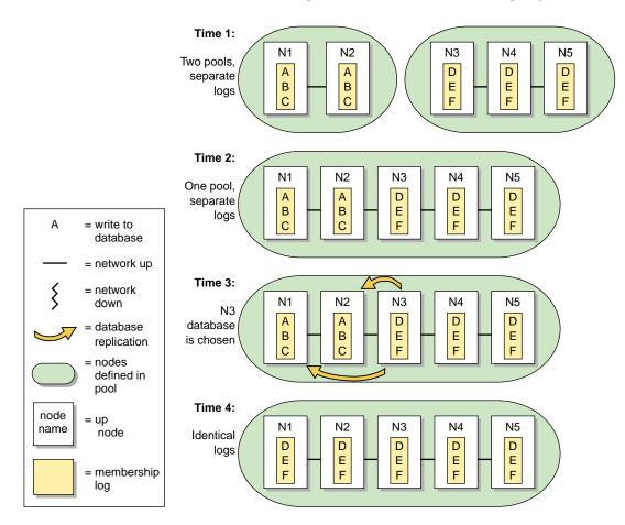
Figure 5-2 Unequally Sized Pools are Joined: Larger Pool Log is Replicated
