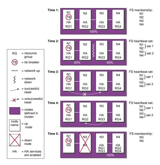
Figure 5-6 Forming a Membership without the FailSafe Tiebreaker
