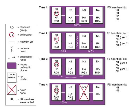
Figure 5-5 FailSafe Tiebreaker Node
