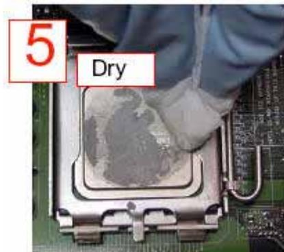
5. Use a different lint-free cloth moistened with isopropyl alcohol (IPA) to remove any remaining TIM from the processor.
