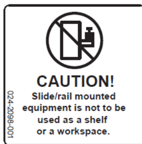
Figure 2-1 Slide/Rail Equipment Usage Caution
