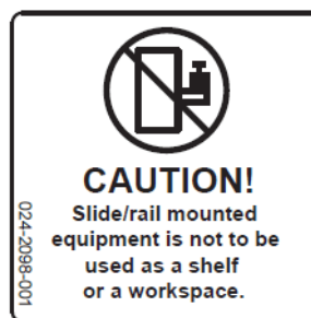
Figure 2-2 Improper Use of Server Rack and Railing
