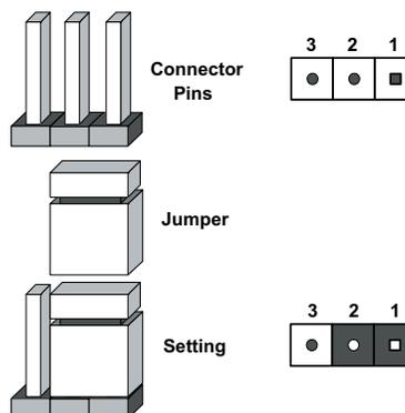
**Note:** On two-pin jumpers, "Closed" means the jumper is on and "Open" means the jumper is off the pins.
